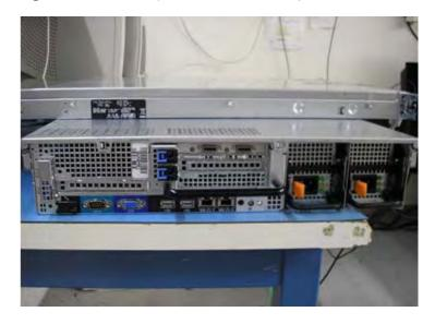
Figure 2. VOD 125/300W (Dell 2950 – Rear View)
